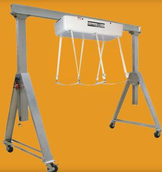
This lift is stationary when mounted parallel to the i-beam of the gantry. track may be added to move the lift from side to side on the gantry. The gantry can also be moved around the room by using a gantry fitted with casters.
