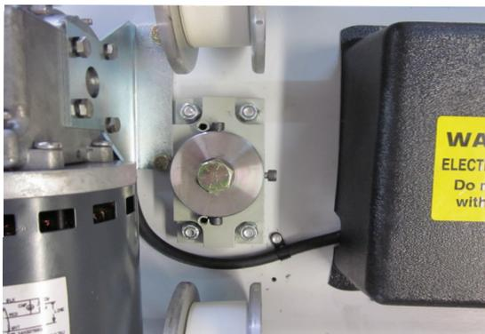
8. Once you have the machine centered on the trolley screw in the 5/8 - 13x4" pivot bolt and tighten down.
